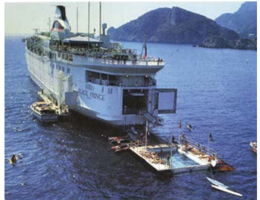
The Black Prince showing the marina floated out from her stern (Photo AnthonCooke)
